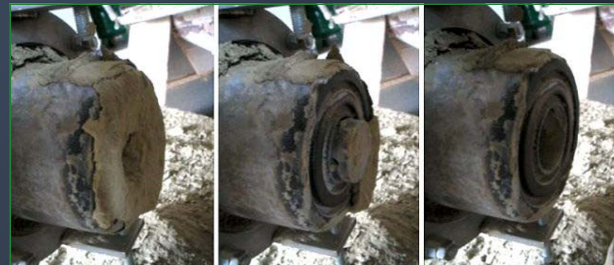
The mechanical cleaning in time succession (Duration approx. 2 s)
